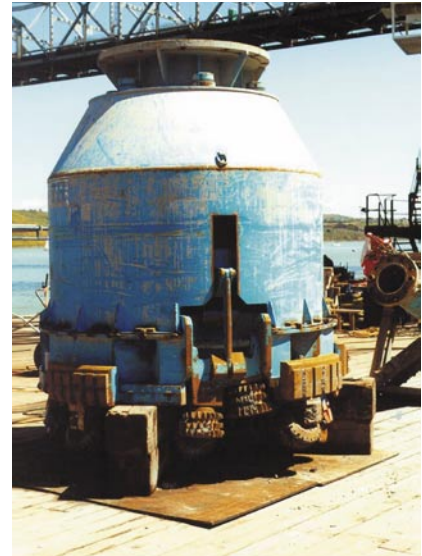
Large-diameter internal drill.
