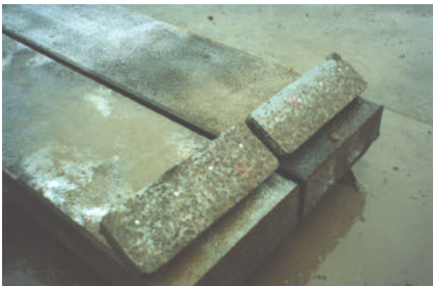
Figure 4. Lightweight concrete specimens from large-scale precast constructibility test were saw-cut. The upper specimen showing segregation due to overdosing of chemical admixtures, the lower specimen showing uniform distribution of aggregates when concrete is properly mixed.
