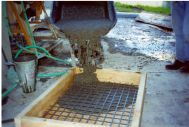
Figure 2. A Small-scale constructibility test of self-compacting concrete
