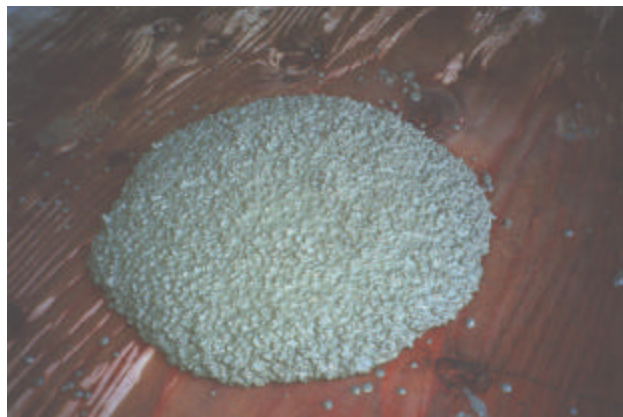
Figure 1. Concrete slump flow in the range of 460 mm to 560 mm
