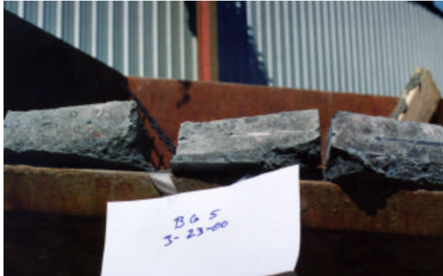
Figure 3. Specimens were cut to show uniform aggregates distribution
