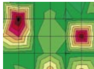
Localised corrosion of red areas.
